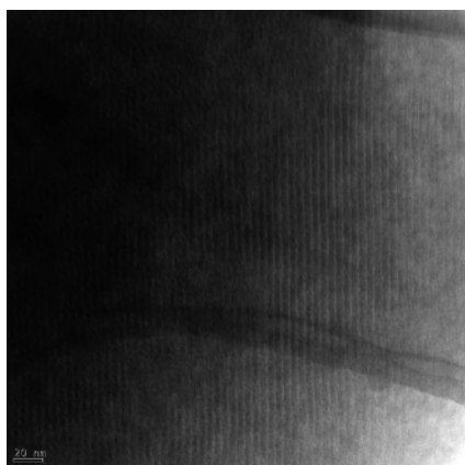
Figure 6. TEM image of carbon monolith, C-15-60, with a hexagonal mesostructure.
